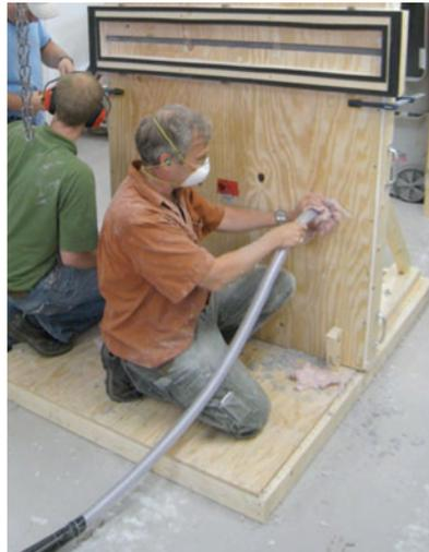
**Photograph 2: Skunk Works Air Leakage Testing**—They only work this hard when we have a camera and the boss is around. A test wall cavity is being insulated with “dense pack” insulation.
