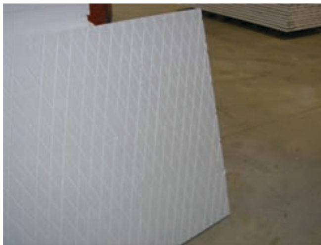
Photograph 5: “Groovy” - Cutting grooves into the continuous insulation to facilitate drainage also provides redistribution of moisture.
