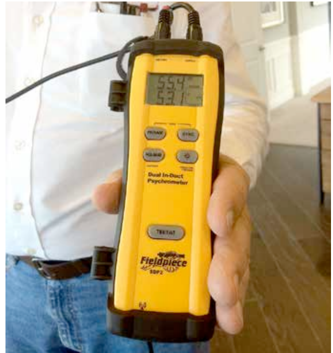
Photograph 11: Meter Reading —Have a camera ready to record for posterity his proof of just how wrong you are. Oops. Not wrong. Meter must be wrong. Actually, no. Difference in dewpoint temperatures between floor and ceiling.
